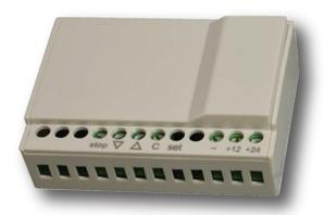
Contact closure interfaces allows integration of the Automation© systems throughout the house. The contact closure interface communicates to LuXout Shades via ARC™ RF communication. Each interface can control one group or one shade using two conductor - one pair #18 AWG (1.0mm<sup>2</sup>), class 2 cable.
