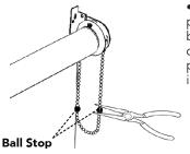
• On the opposite side, place a ball stop on the bead closest to the clutch. Use needle nose pliers to clamp ball stop in place.
